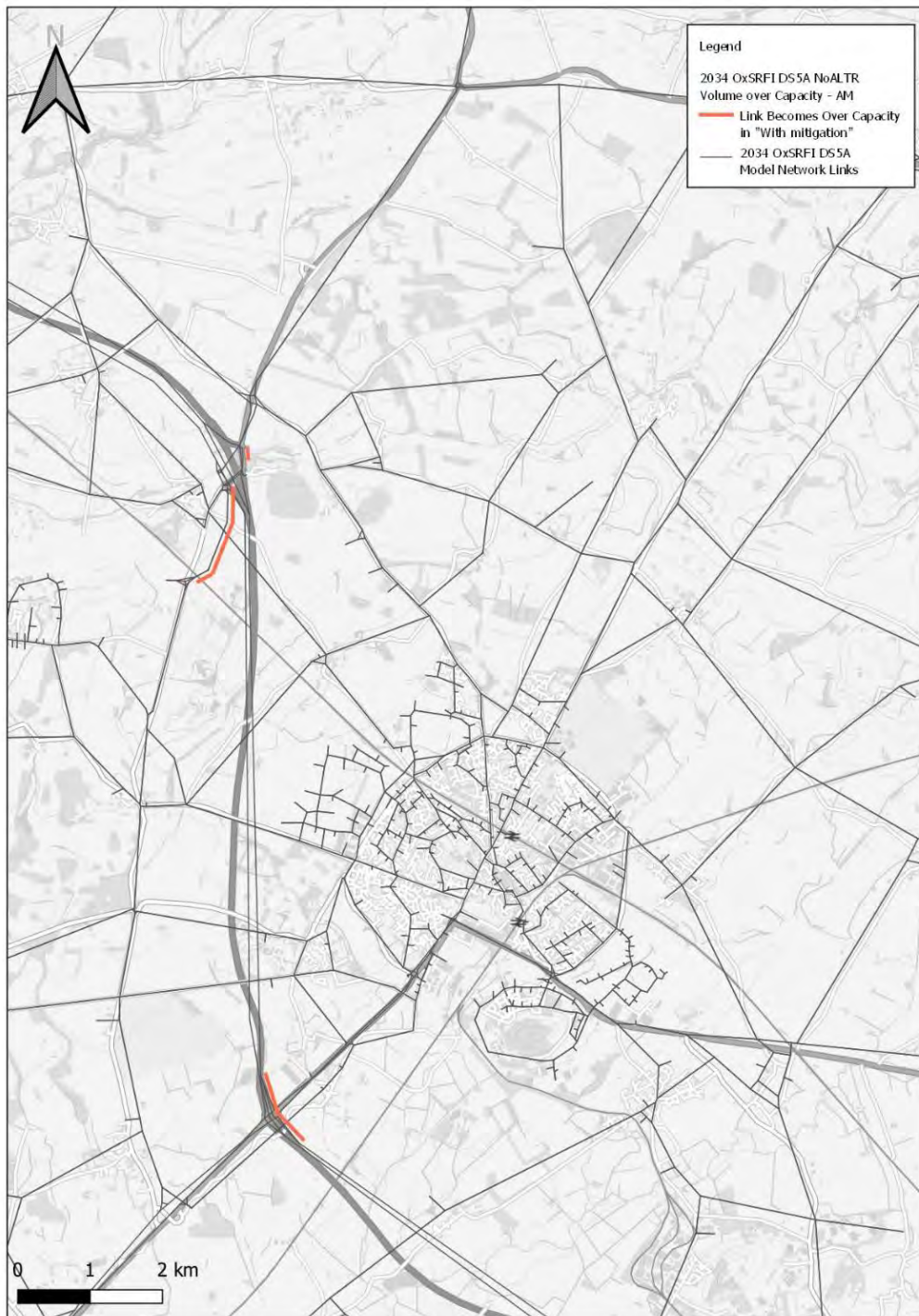
Figure 5-12 : 2034 AM links where volume exceeds 85% capacity in the Do Something scenario and not the Do Minimum. Scenario 8 - Scenario 7
