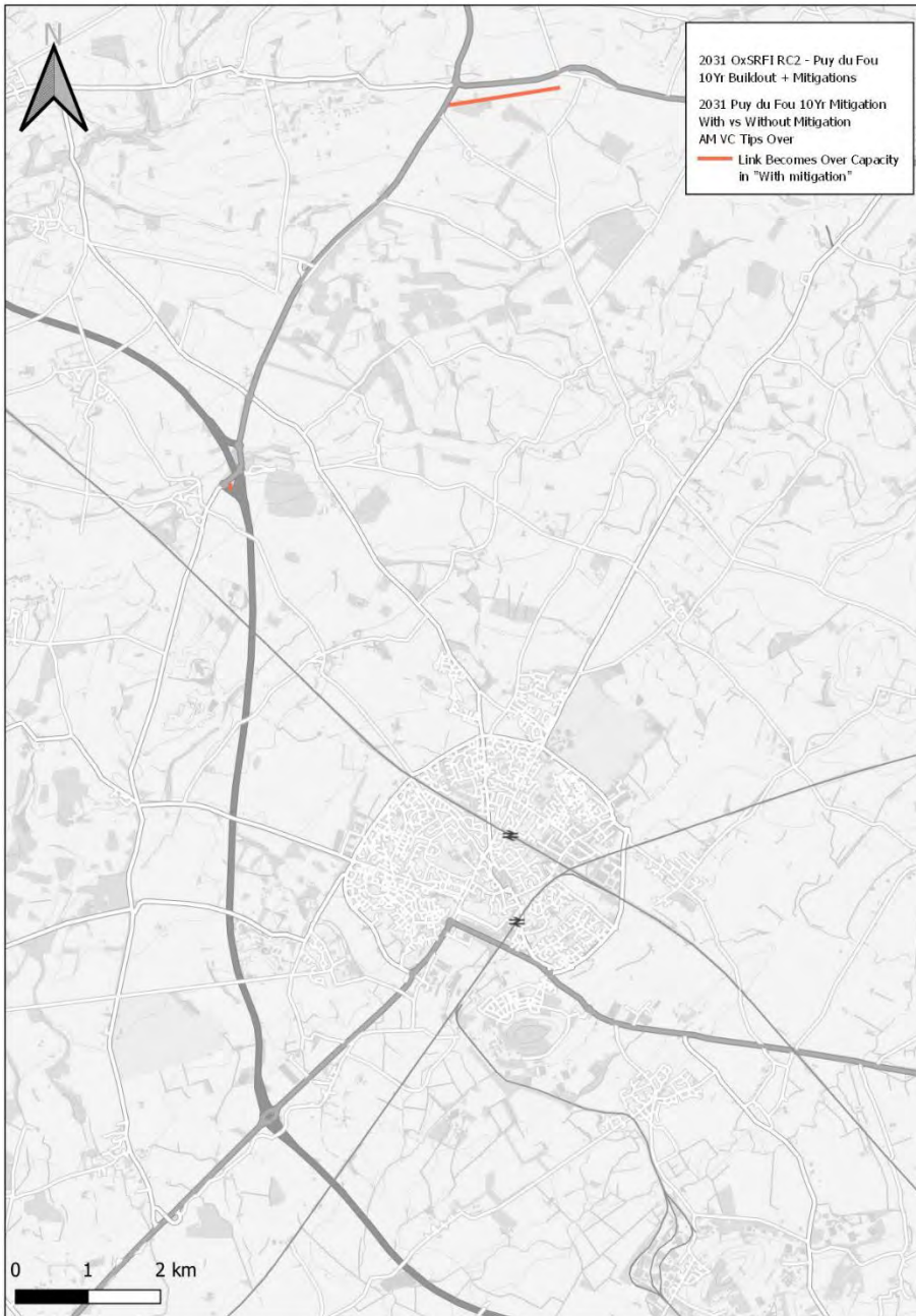
Figure 5-6 : 2031 AM links where volume exceeds 85% capacity in the Do Something scenario and not the Do Minimum. Scenario 6 - Scenario 5
