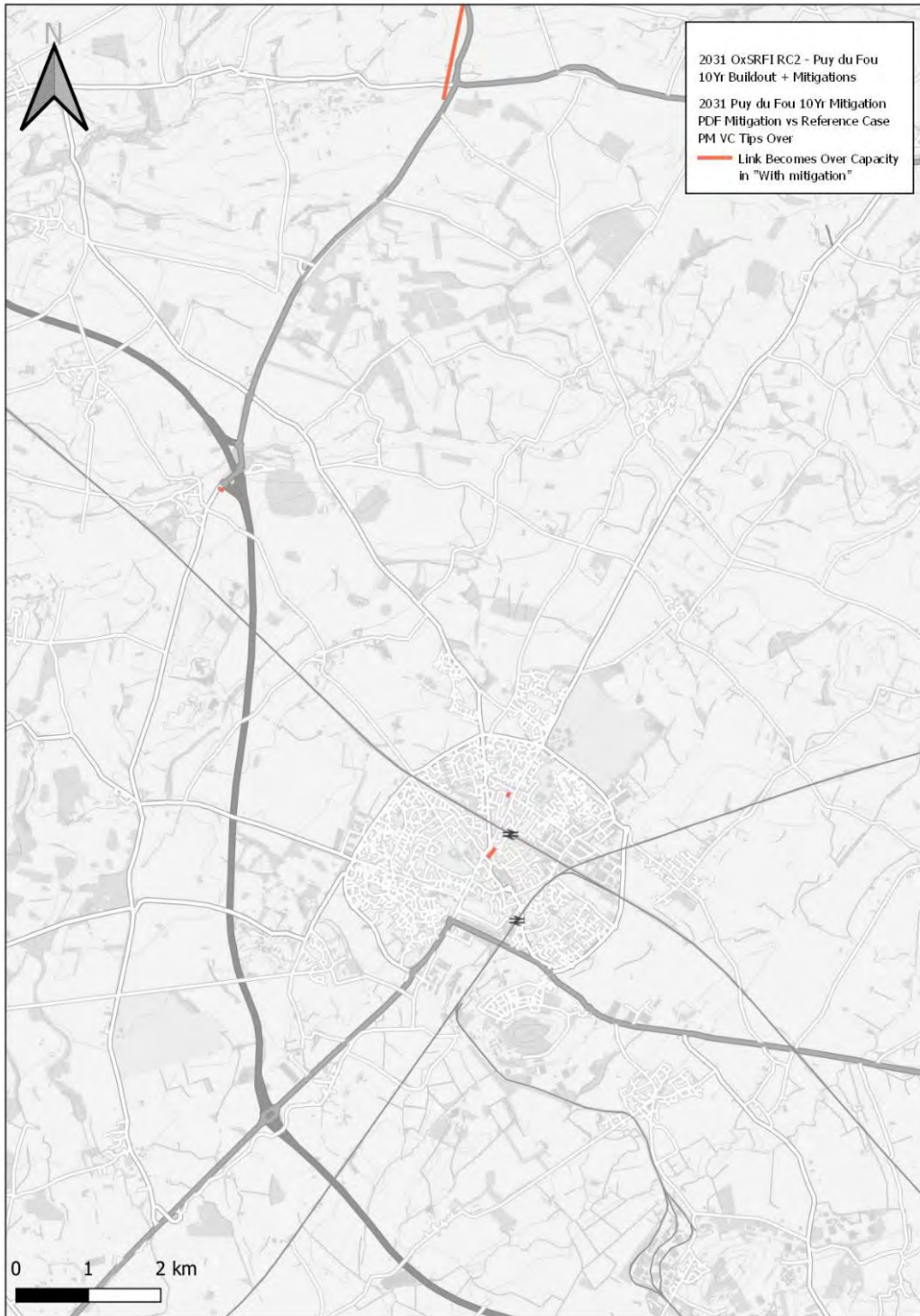
Figure 5-19 : 2031 AM links where volume exceeds 85% capacity in the Do Something scenario and not the Do Minimum. Scenario 6 – 2031 RC
