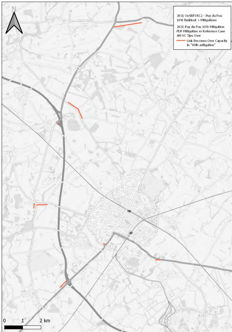
Figure 5-18 : 2031 AM links where volume exceeds 85% capacity in the Do Something scenario and not the Do Minimum. Scenario 6 - Scenario 5
