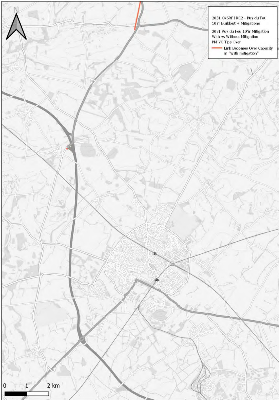
Figure 5-7 : 2031 AM links where volume exceeds 85% capacity in the Do Something scenario and not the Do Minimum. Scenario 6 - Scenario 5
